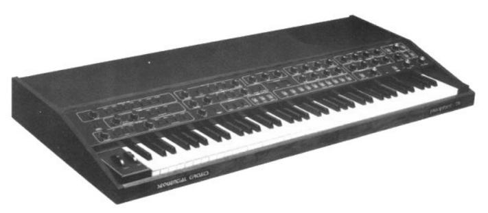
Sequential Circuits has done it again! Introducing the **PROPHET- T8**: a completely touch sensitive (velocity and pressure), fully programmable, 8-voice polyphonic synthesizer! The 76-note wooden keyboard (A to Q has been packaged in a compact design weighing less than 60 lbs. and measuring 48" long, 21" deep, and a scant41/2" high. With 128 programs, this instrument is the most sophisticated 8-voice synthesizer ever.
